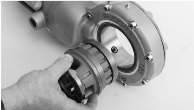
Figure 4 – Installing Die Heads into 700 Power Drive
