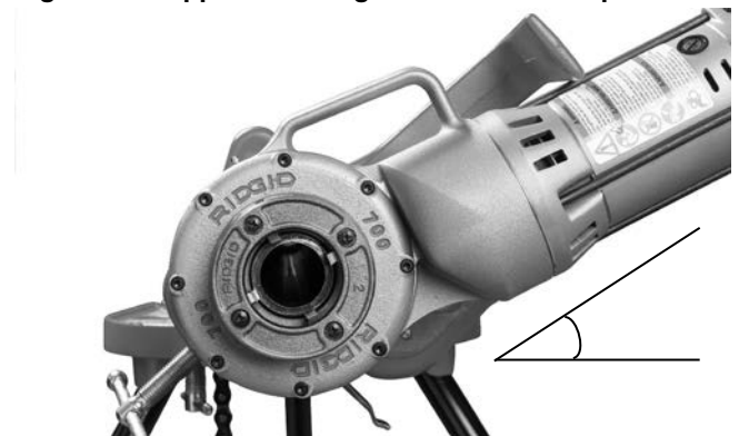
Figure 6 – Support Arm Positioned With 700 Power Drive Slightly Above Horizontal
